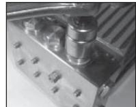
5) Tighten up tension plugs (48) to 107 ft.-lbs.
