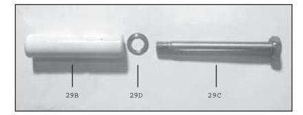
12) Check plurger surface (29B). If plurger pipe is worn out, loosen tension screws (29C) with a 15mm socket and pull off plurger pipe to the front. Clean front surface of plurger (29B) thoroughly.Apply a small drop of locktite to tension screw. Rt a new crush washer (29D) onto tension screw. Rt a thin cost of glue (loctite) on the ring (or ceramic plurger side) and tighten screw to 265 in.-lbs.
