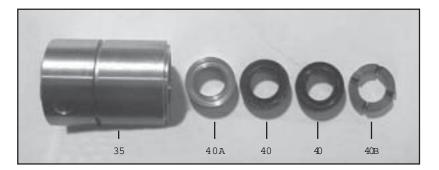
11) Remove the pressure ring (40A), v-sleeves (40), and support ring (40B), from the seal sleeve. For LP301A and LP301A-4000 pumps, remove the pressure spring (41). Examine seals carefully and replace if worn. Clean surfaces of seal sleeves (35) which come in contact with the crankcase (1) and sealing surfaces of valve casing (43).
