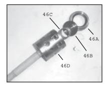
4) Loosen value seats (46A) and value spring (46C) from spacer pipe (46D) by lightly hitting the value plate (46B) with a plastic stick. Check sealing surface and replace worn parts. Reassenble with new o-rings (44A) if possible and oil them before installing.
