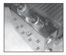
3) Take out discharge value assentblies (46) by pulling them upwards out of the value casing (43) with a snap-ring tongs or any other pull-off device. Then remove inlet values in the same way.
